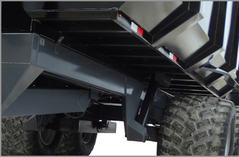
Weight Transferring Tandem 8% less weight on front axle and tires for less turn scuffs on crops, less tire wear, and better flotation.
